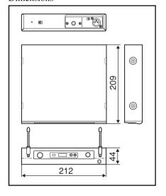
$212 \times 44 \times 209 \text{ mm } (8^{3}/8 \times 1^{3}/4 \times 8^{1}/4 \text{ inches) } (\text{w/h/d})$  (excluding the antennas)
